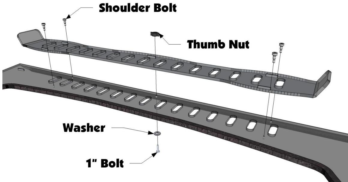
6. Now you are ready to place the windshield on the vehicle. With assistance, place the upper windshield on the frame. Wrap the clamps provided around the steel frame tubing at all slot locations. Now place the bolts and washers through the slots with washers on the inside of the windshield on top of the clamps. Run the bolts through the clamps on the backside, and install a thumbnut on the outside of the windshield to secure. Repeat with the lower windshield. See Diagram Below.
