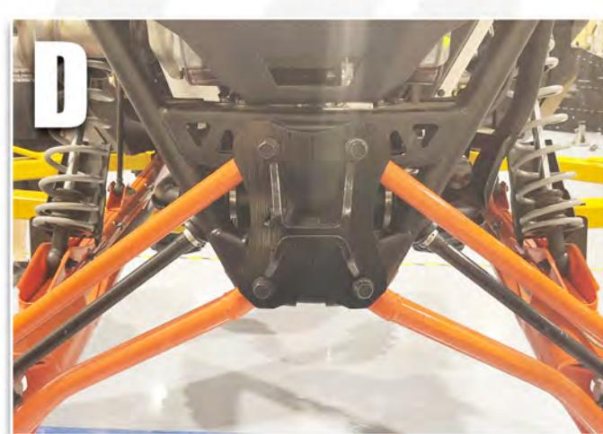
CHECK TO SEE THAT EVERYTHING FITS THEN TIGHTEN BOLTS TO FACTORY SPECS. REINSTALL WHEELS AND LOWER THE JACK.
